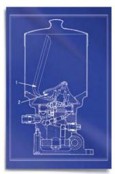
Figure 7. Multi-outlet lubricator with grease vane (1) and pre-feed roller (2). The roller forces the grease into the suction cavity. This unique design can handle greases up to NLGI Class 4.
