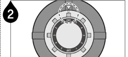
2 Set the control knob to 'OFF' position before filling the lubricator.
