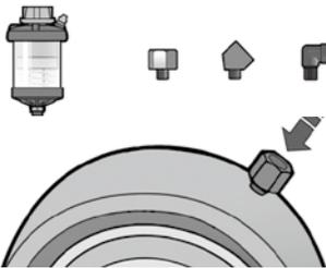
The Pulsarlube S is designed for single point lubrication only. Direct mount is always preferable.
