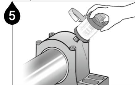
5 Install the PulsarLube S unit on the lube point.
