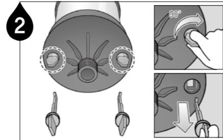
2 Turn and pull out the piston clamps found at the bottom of the lubricator.
