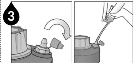
3 Remove the red grease cap and fill lubricator until the piston ring reaches level indicator line that reads "Do not fill below this line". Refer to the grease filling information on the back.
