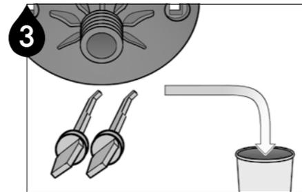
3 Dispose of the piston clamps removed from the lubricator.
