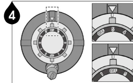
4 Turn the control knob to #5 to make sure the lubricator is dispensing properly. After checking, turn the control knob back to 'OFF' position.
