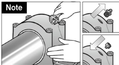
**Note** Remove the grease nipple and install appropriate adaptors.
