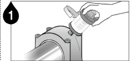
1 Install the PulsarLube S unit on the lube point for easy filling of grease.
