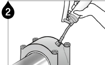
2 Ensure a clear passage using a manual grease gun. **Note 1** Remove any hardened grease by purging the lube point with a manual grease gun. **Note 2** The grease in the equipment and the grease contained in the unit should be the same or compatible.
