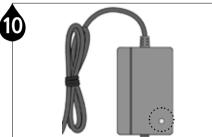
Converter turns on when the control panel powers on.
