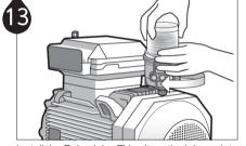
Install the Pulsarlube EX unit on the lube point.
