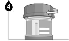
Put the cap back on and turn it clockwise until the cap is securely locked in place.
