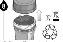
The Pulsarlube EO is an eco-friendly product that can be recycled. Turn the housing cap counterclockwise to disassemble the product for proper disposal.
