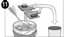
Using a hand tool such as a flat-head screwdriver, detach the PCB from the unit.
