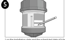
Log the installation date and the scheduled date of lube cycle completion on the label of the Pulsarlube EO. Note Please note there is a delay before the unit starts dispensing oil. It can take up to 3 weeks for enough gas to generate to start dispensing
