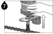
When the selected dispensing period of the Pulsarlube EO has completed, remove the lubricator from the application.
