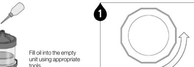
Turn the housing cap counterclockwise to unscrew the cap.
