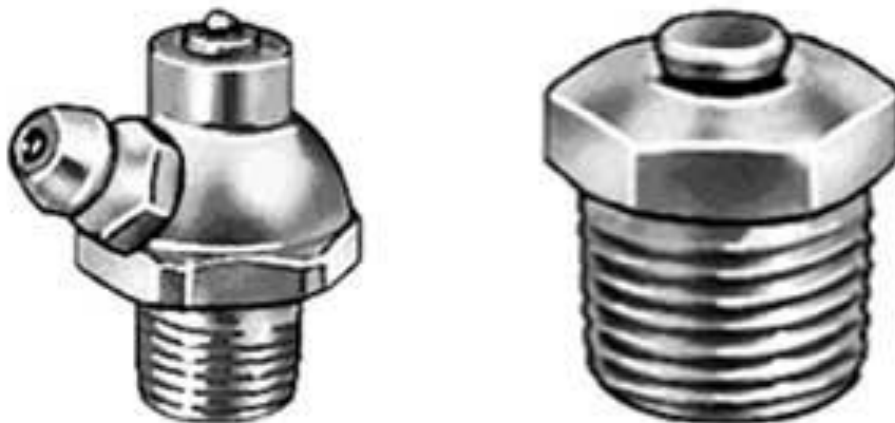
Figure 9. The pressure cut-off-fill-plug does not allow additional grease to be added to a grease cavity when the pressure exceeds 20 psi. (Left)
